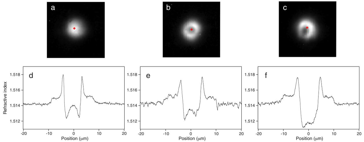
Figure 1: Waveguide evaluation. Frames a, b, c, show the near-field mode of 1550 nm laser light coupled into waveguides fabricated by translating the sample at 20 mm/s, 10 mm/s and 5 mm/s, respectively (cross shows mode centroid). Frames d, e, f show refractive index profiles obtained using the refractive near-field technique of each of these waveguides. Single mode propagation is obtained with the waveguides made at 20 mm/s, where the central bump in the index is most pronounced.
