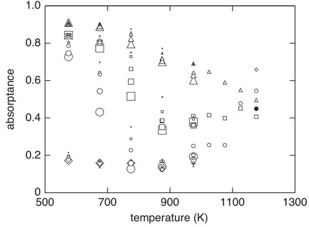
FIG. 3: Average absorptance from 1250–2500 nm for sulfur-doped (circles), selenium-doped (squares), tellurium-doped (triangles) silicon and samples irradiated in N<sub>2</sub> (diamonds) after various thermal anneals at  $T \leq 975$  K. A larger marker indicates a longer anneal (from smallest to largest: 10 min, 30 min, 100 min, 6 h, 24 h).
