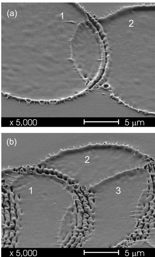
FIG. 2. SEM images of crater rims generated by overlapping laser pulses (a) two pulses and (b) three pulses of 800 nm and 100 fs. The laser fluence was  $F_0 = 0.34 \text{ J/mm}^2$ . The numbers correspond to the order of the incident laser pulses.
