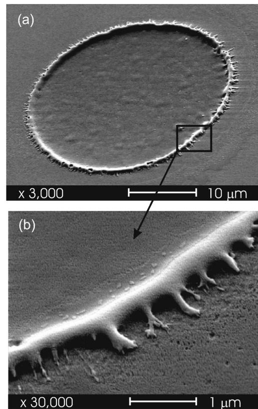
FIG. 3. SEM images of a crater generated with a single 800 nm and 100 fs laser pulse. (a) The whole crater at  $3000\times$  magnification and (b) a higher resolution SEM image ( $30\,000\times$  magnification) focused on the rim formed around the crater. The laser fluence was  $F_0 = 0.34 \text{ J/mm}^2$ .
