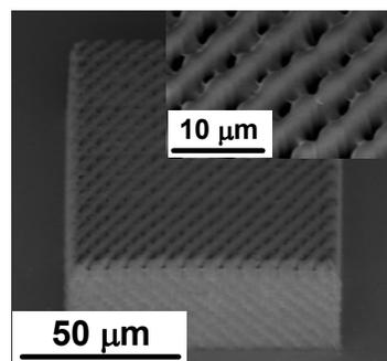
**Figure 3** - Scanning electron micrograph of an interconnected structure for biological applications. The inset shows a detail of the structure.
