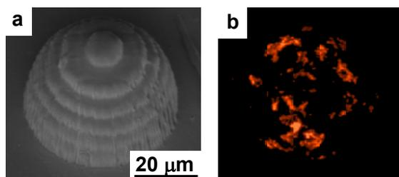
**Figure 2** – a: Scanning electron micrograph of the polymeric blend containing the acrylic-based resin and MEH-PPV. b: fluorescence microscopy of the polymeric blend.
