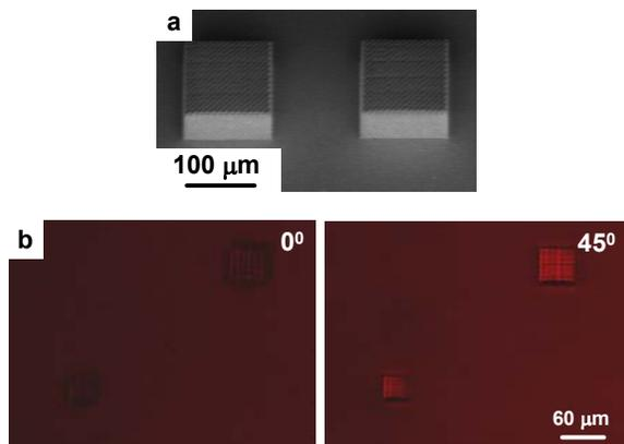
**Figure 1** – a: Scanning electron micrograph of solid squares structure fabricated by 2PA polymerization. b: Polarization microscopy for sample like the ones shown in a. The angle between the polarizer and sample is shown in the top right corner of each image.
