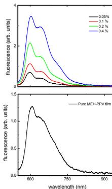
This figure shows the fluorescence spectra of thin films prepared with pure MEH-PPV and the polymeric blend with the acrylate resin. For excitation we used an Ar ion laser operating at 514 nm.
