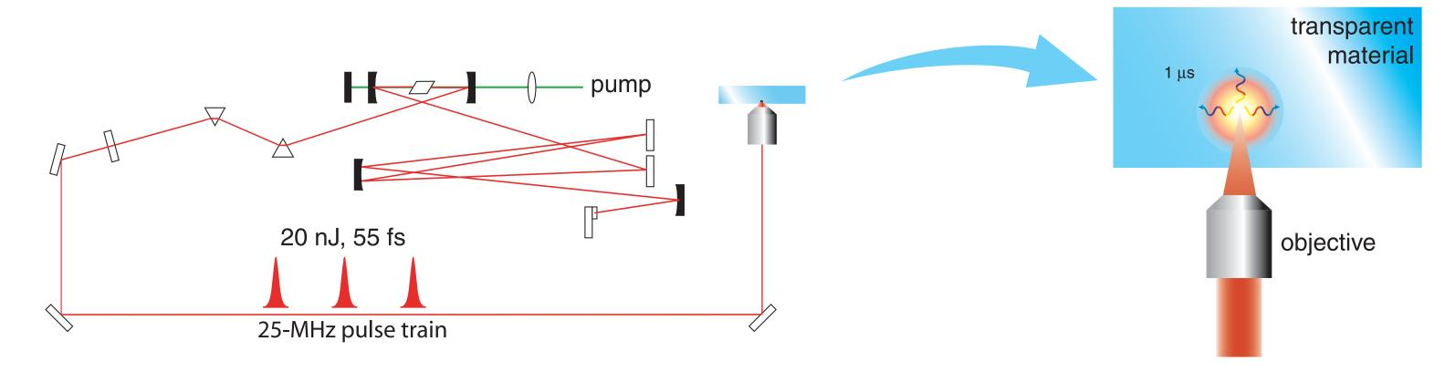
By extending the cavity of a standard Ti:sapphire laser oscillator, we generate a 25-MHz pulse train of 20-nJ pulses — enough energy to produce nonlinear absorption.
