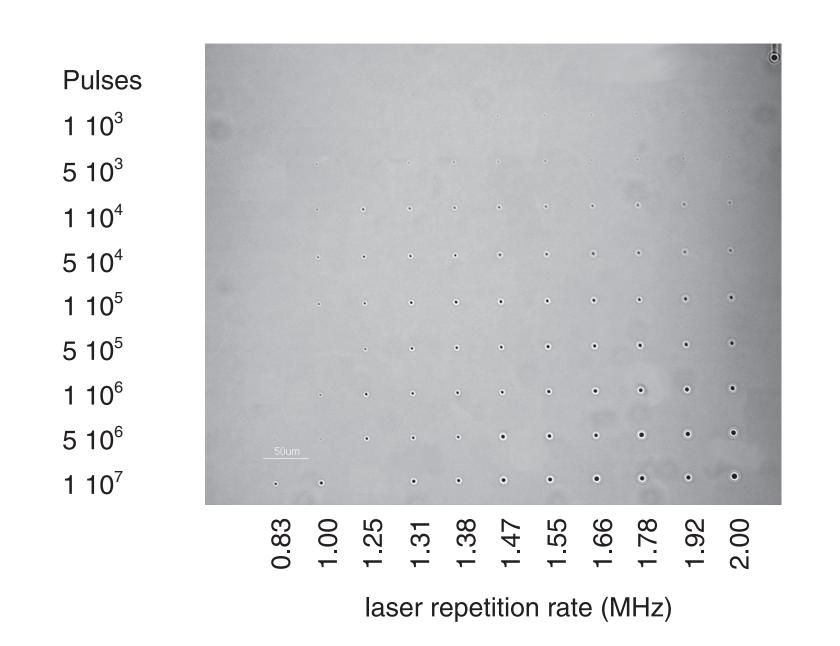
Corning 0215 slide irradiated with increasing number of laser pulses per spot at different repetition rates. For low number of laser pulses modification still occurs. The number of pulses inside each laser packet is equal to 10. Individual laser pulse energy is constant throughout (1.4 N.A. focusing).
