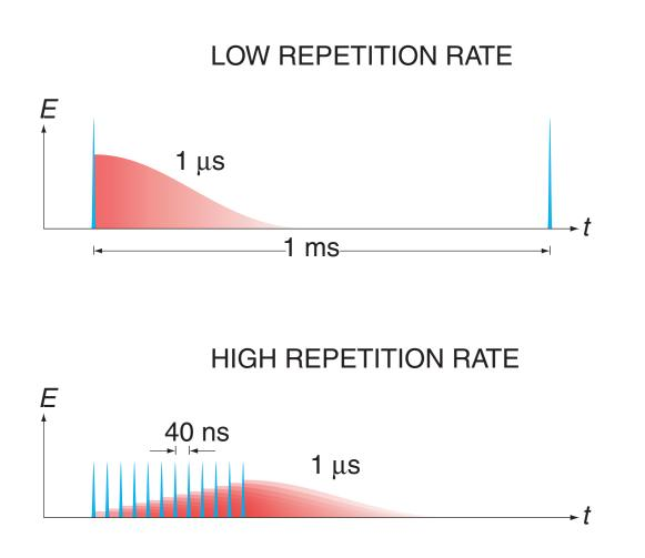
Energy deposition by an amplified laser system (1 kHz) and by an oscillator (25 MHz). Yellow indicates optical pulses and red indicates thermal energy.
