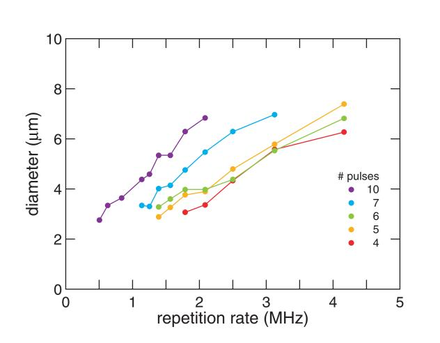
Repetition rate dependence of the waveguide diameter in Corning 0215 for various number of pulses in packet.. Pulse energy at sample is maintained at 5.5 nJ, focusing 1.4 numerical aperture lens, translation speed 1 mm/s.
