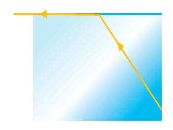
At the 'critical angle', the bent ray travels along the surface
