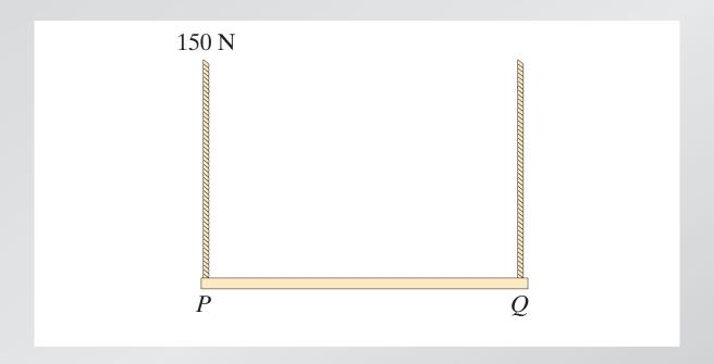
A uniform plank is supported by two ropes at points *P* and *Q*. The tension in the rope at *P* is 150 N.
