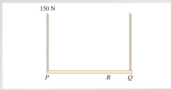
A uniform plank is supported by two ropes at points *P* and *Q*. The tension in the rope at *P* is 150 N. The point at which the other rope is attached to the plank is now moved to point *R* halfway between Q and the center of the plank. What are the tensions in the two ropes?
