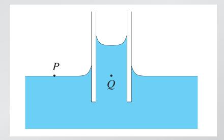
1. Consider the capillary rise of a liquid in a glass tube. How does the pressure at point *P* at the surface of the liquid compare to the pressure at point *Q* at equal height?
