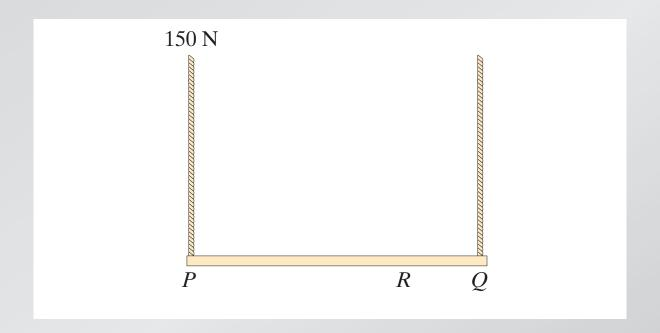
A uniform plank is supported by two ropes at points *P* and *Q*. The tension in the rope at *P* is 150 N. The point at which the other rope is attached to the plank is now moved to point *R* halfway between Q and the center of the plank. What are the tensions in the two ropes?
