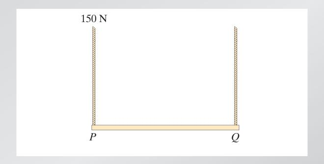
A uniform plank is supported by two ropes at points *P* and *Q*. The tension in the rope at *P* is 150 N.
