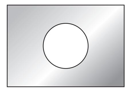
Consider a metal (aluminum) plate with a hole in it. If you heat the plate uniformly what happens to diameter of hole?
