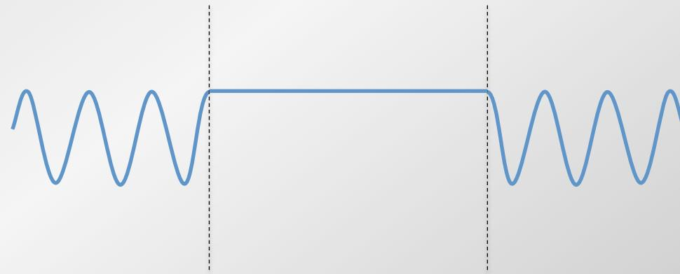
at zero index, wavelength and phase velocity become **infinite**
