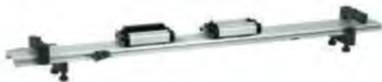
Figure 4.2 Low-friction track and carts used in the experiments described in this chapter.
