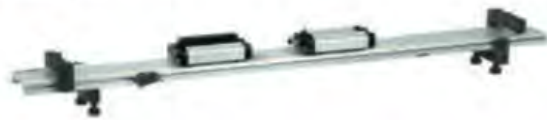
Figure 4.2 Low-friction track and carts used in the experiments described in this chapter.
