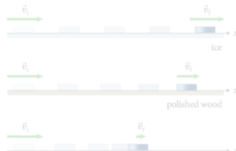
Figure 4.1 Velocity-versus-time graph for a wooden block sliding on three different surfaces. The rougher the surface, the more quickly the velocity decreases.
