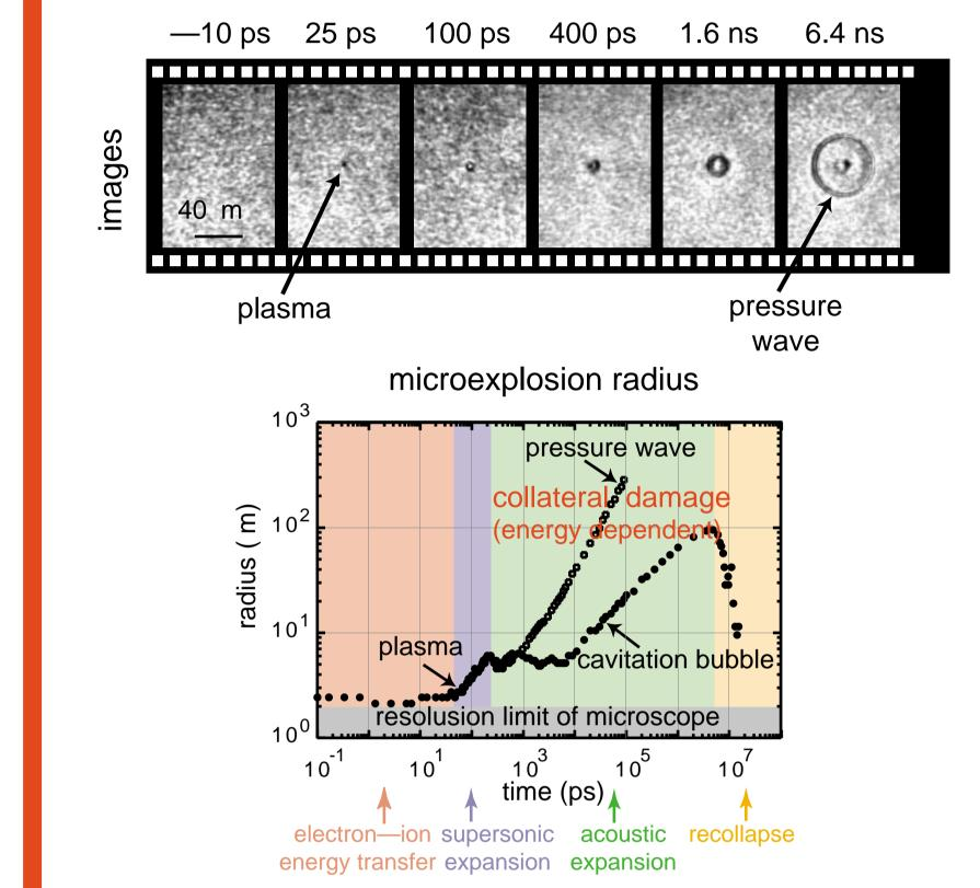
Femtosecond pulses minimize collateral damage in biological samples.
